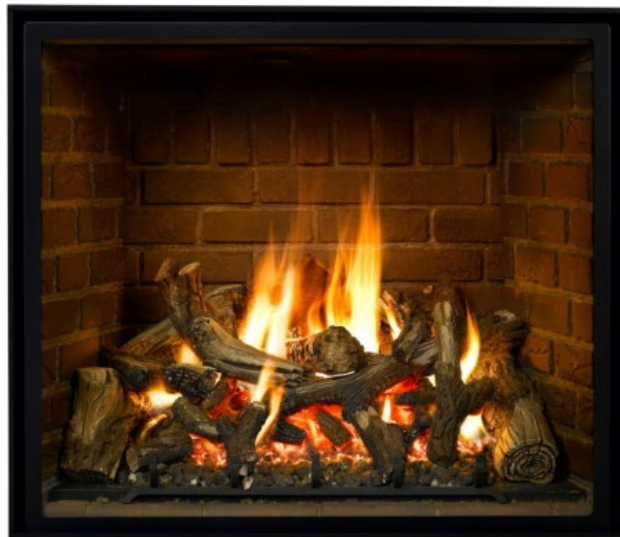
Figure 6-2 Burner Flame Heights: This image provides a visual reference for the burner flames burning at maximum height after the burners have been operating for 30 minutes or longer. A normal rear flame will be 1 to 2 inches above the rear log top edge. This, however, is dependent on the gas type, air shutter opening setting and vent system configuration. Actual flame heights can be slightly higher or lower when compared to this reference image.
